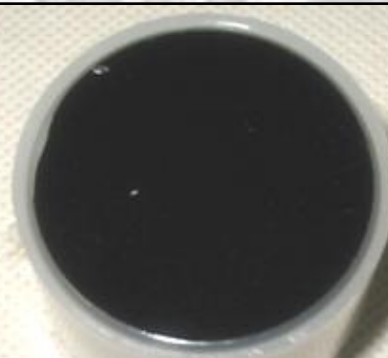
Bottom View of Sample in Liquid XRF Cup
